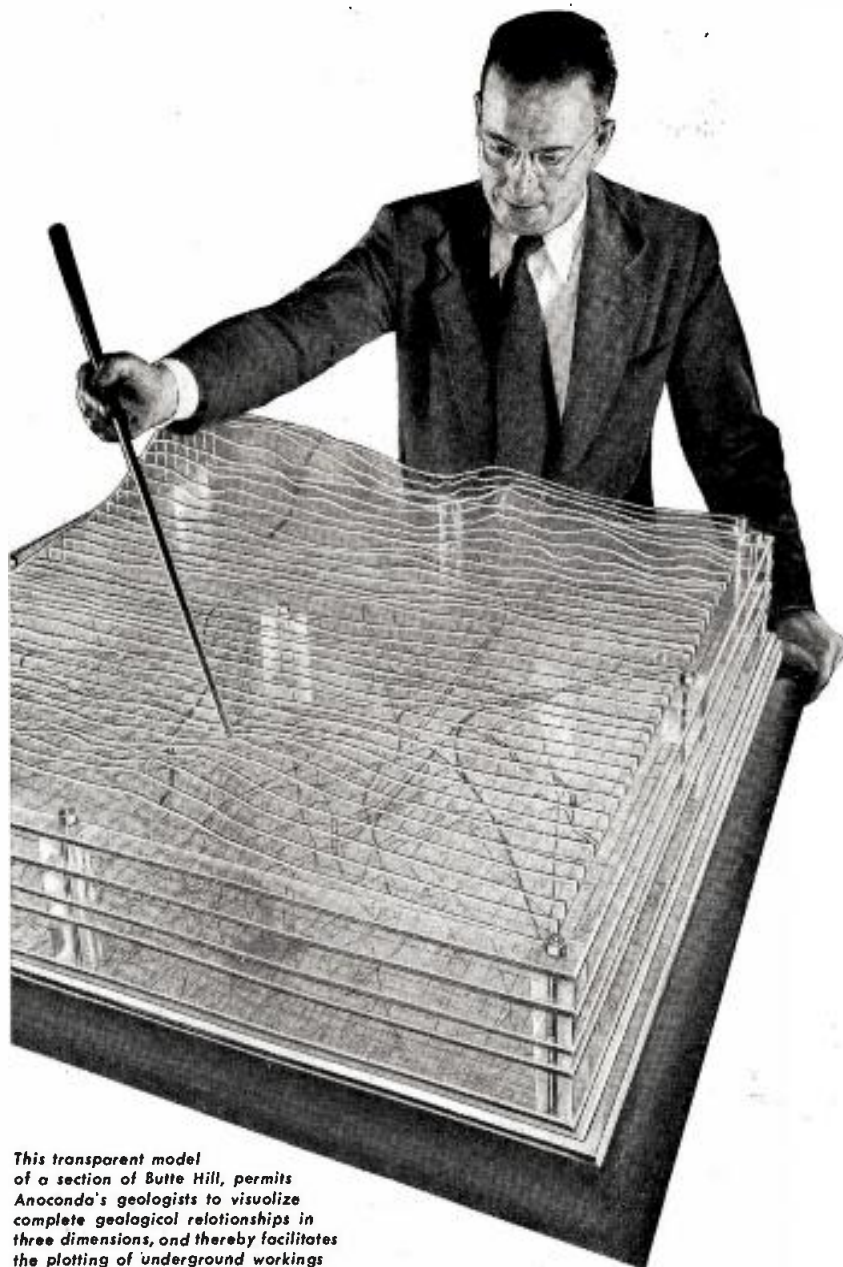
The construction and study of scale mine models such as this provide valuable geological information for mine development.
